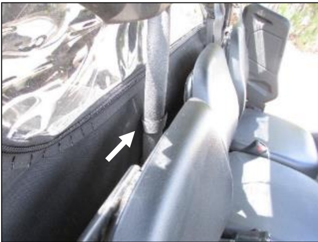
17. Secure the back panel with two Velcro loops around the rear pillars of the cab. There is one behind the passenger and drivers seats.
