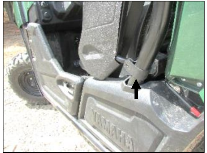
4. Attach a clamp in the rear upright bar as shown above
