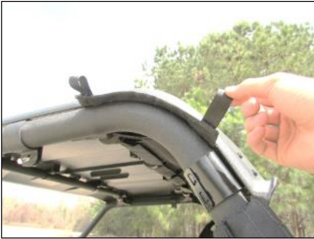
15. Pull the loop through the side of the vehicle between the roll cage and roof.
