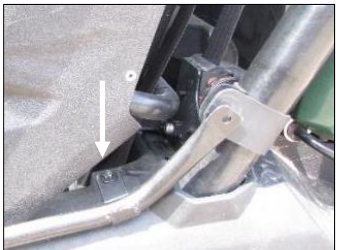
8. Remove the bolt behind the seat and use to install the Z bracket.
